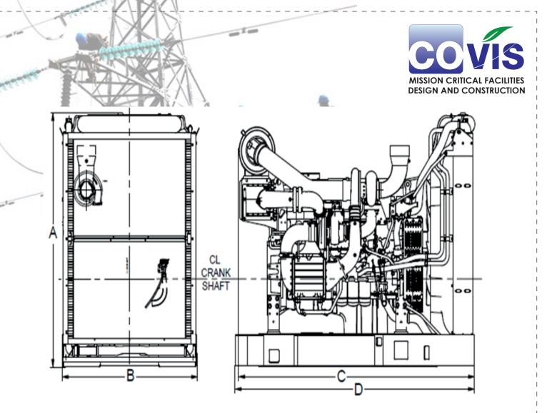
$A^* = 1930 \text{ mm} / 76 \text{ in}$   $B^* = 1350 \text{ mm} / 53.1 \text{ in}$  C = 2362 mm / 93 in D = 2399 mm / 94.5 in (During Transport) D = Max 3255 mm / 128.2 in\*Including radiator and intercooler
